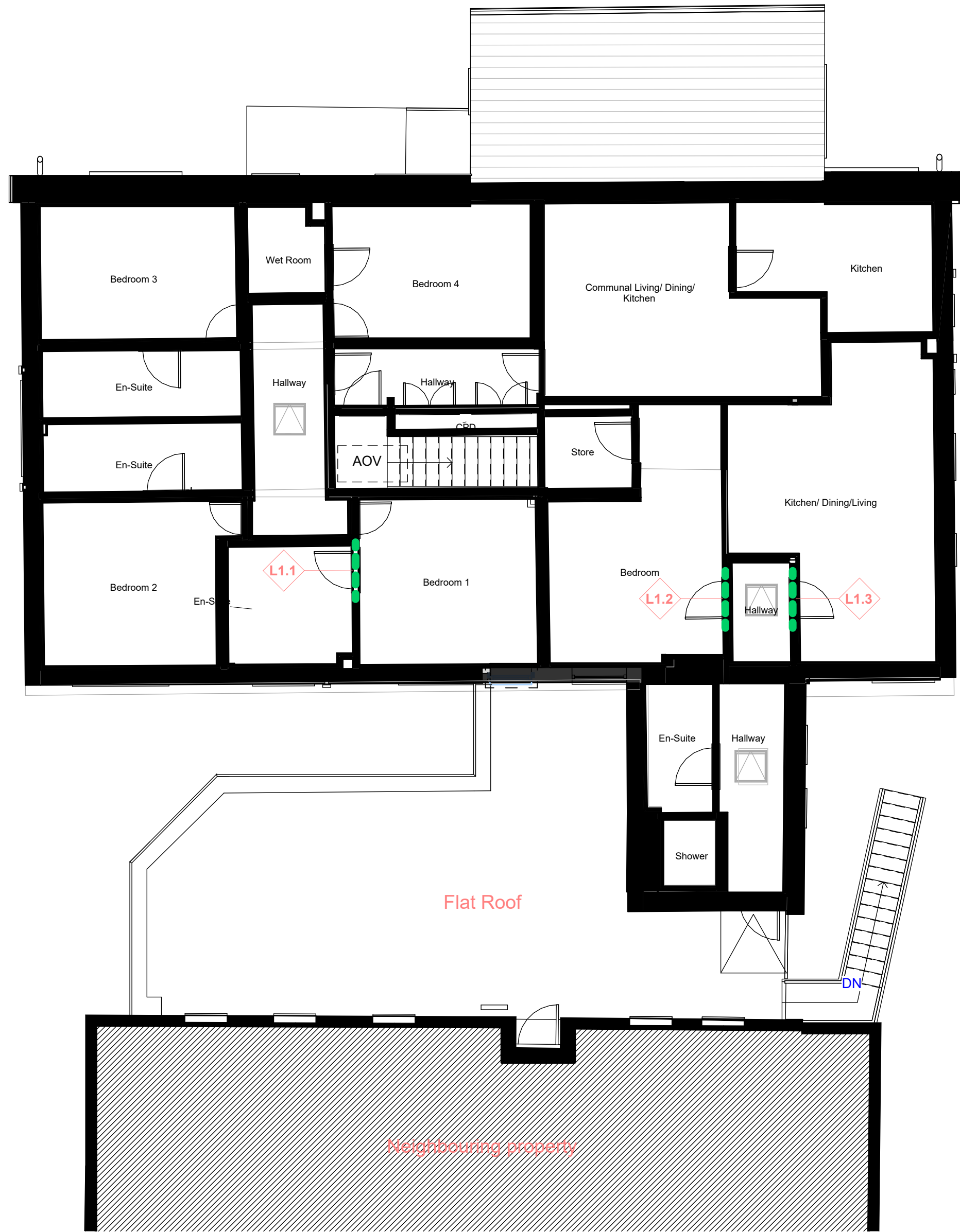
Proposed First Floor Plan - Lintels
